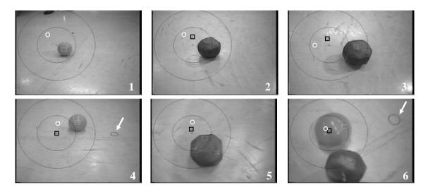
Fig. 14. The robot approaches the goal while avoiding the obstacle. (Views from robot eye)
