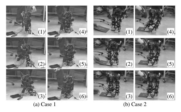
Fig. 8. Actual 'Standing Up' Motion from Leaning Forward and Actual 'Crouching Down' Motion from Stumbling Over a Step
