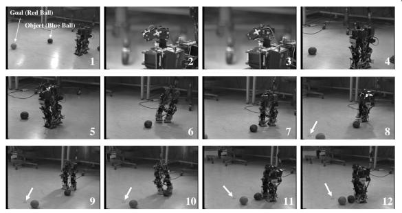
Fig. 13. The robot approaches the goal while avoiding the obstacle. (Views of experimental field)
