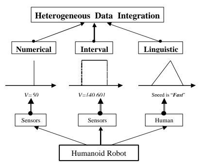
Fig. 2. Example: heterogeneous data integration for the speed measurement of a humanoid robot.
