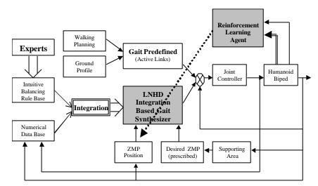
Fig. 8. Humanoid biped gait synthesizing system based on LNHD integration with RL
