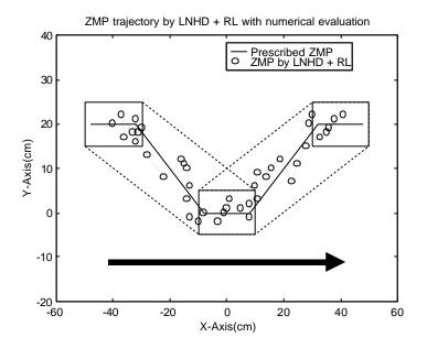
Fig. 10. The ZMP tracing result by RL with numerical evaluative feedback
