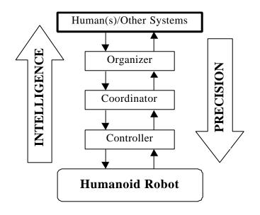
Fig. 1. Hierarchical intelligent robotic control system for a humanoid robot
